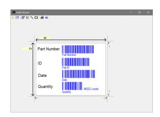
Once a label is designed there is no need to enter the wizard. The design template is applied as required. The active text in the label is updated with the information unique to the part being scanned.
